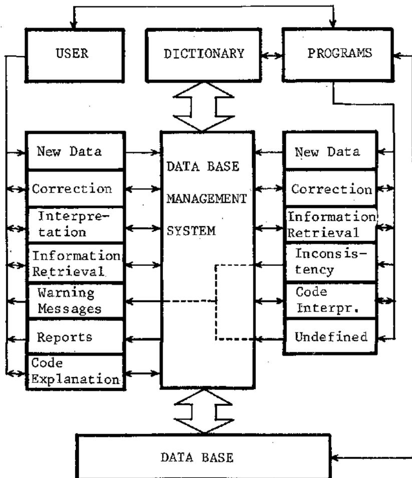
Figure 6. The data management and flow procedures of the software system.
