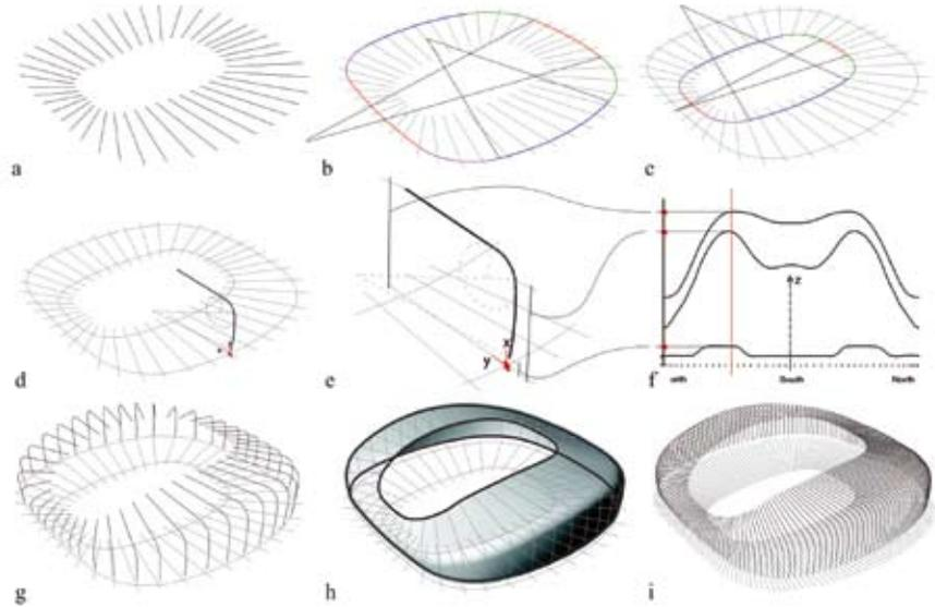
**Figure 4.** The geometric definition of the Aviva Stadium envelope (Shepherd et al., 2011).
