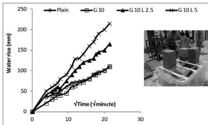
Figure 7. Capillary Water Rise.
