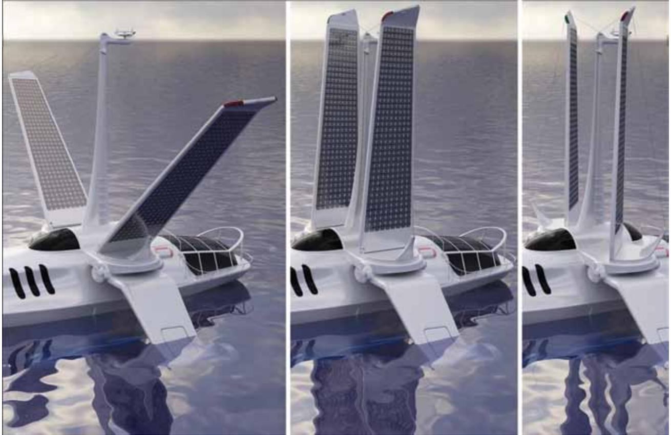
**Figure 7.** Solar Wing Movement Capabilities.
