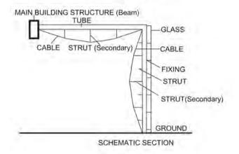
**Figure 2.** SGSPCT with a Distance to the Building (C. Atakara).
