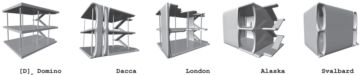
Figure 3. Series of end-products were calculated for different geographic locations through changing the parameters used in the script (such as climatic region, geographic location, sun angle and average temperature).
