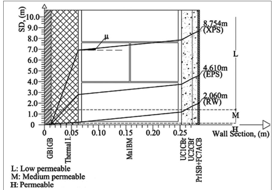
**Figure 9.** The graph showing the increase in total SD value throughout the wall section as a function of layer thickness for the walls internally insulated with RW, EPS or XPS, and externally plastered with FC7ACB. The slope of each line presents the individual  $\mu$  value of each layer.
