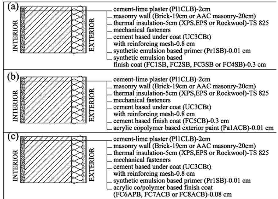
**Figure 2.** Internally insulated single leaf wall plastered with three different finishing composition: (a) synthetic emulsion-based exterior finish coat (FC1SB, FC2SB, FC3SB or FC4SB); (b) cement-based exterior finish coat (FC5CB); (c) acrylic polymer-based exterior finish coat (FC6APB, FC7ACB or FC8ACB).
