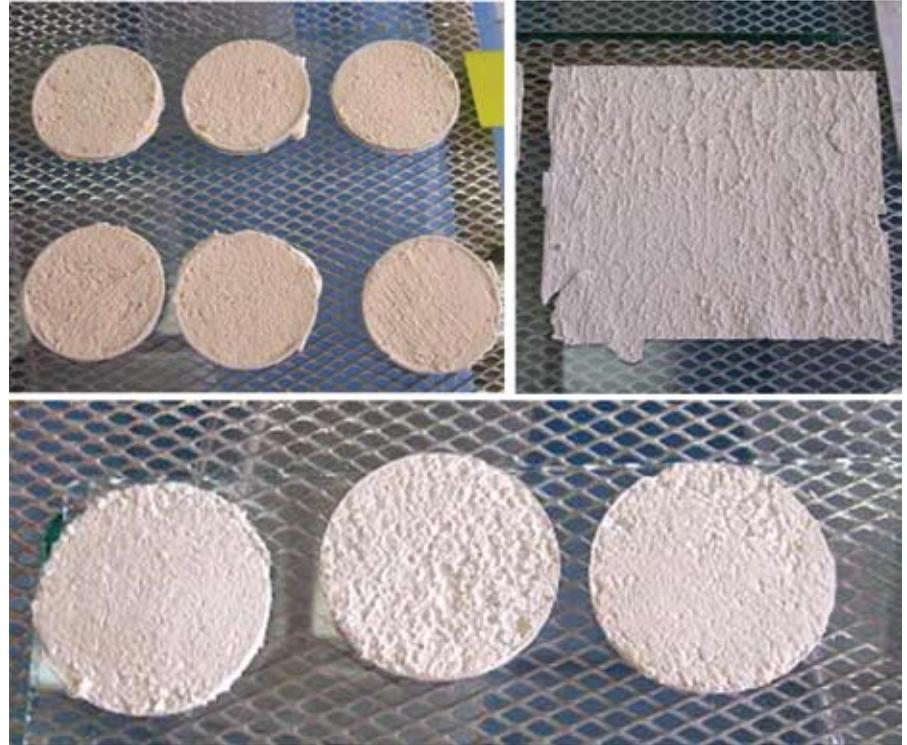
**Figure 3.** The samples: synthetic emulsion-based finish coats with and without primer (at the top left); acrylic polymer-based finish coat applied on primer (at the top right); cement-based finish coat, incorporating a coat of paint (at the bottom).
