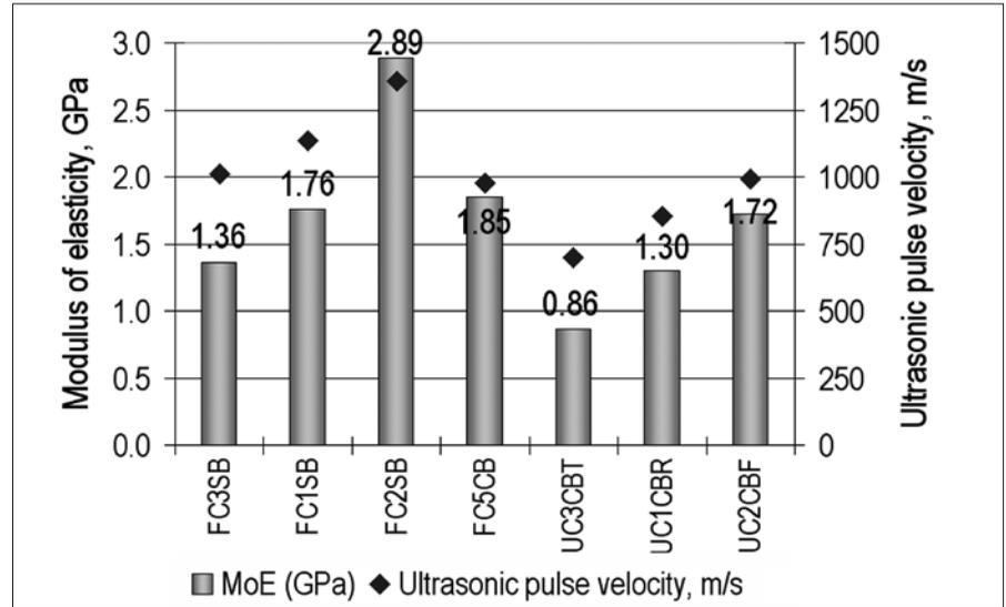
Figure 10. The UPV and MoE values for finish coats and undercoats
