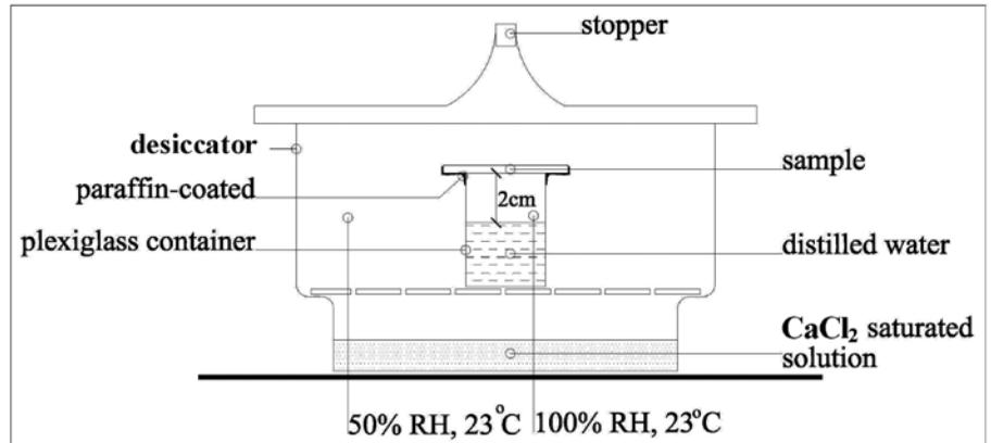
**Figure 4.** The experimental set-up used for the analysis of water vapour permeability properties.
