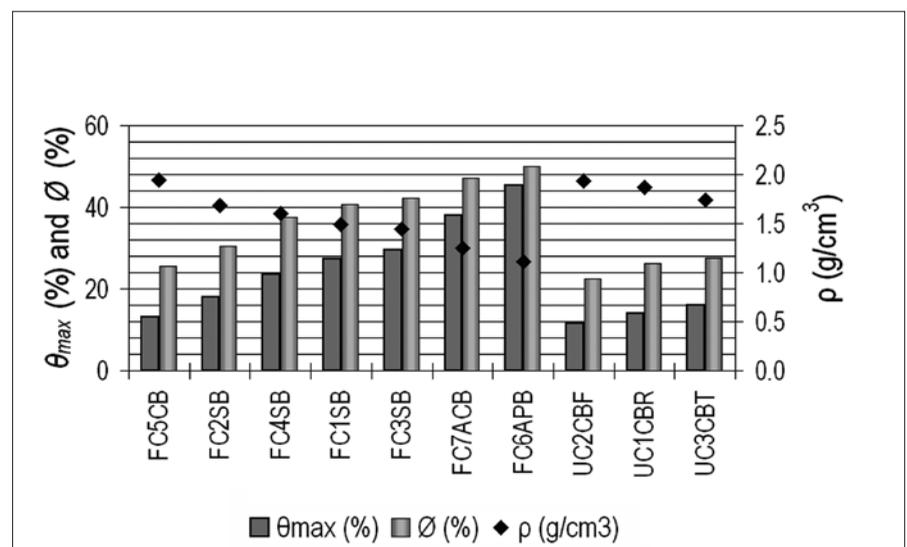
**Figure 5.** The bulk density ( $\rho$ ), porosity ( $\emptyset$ ) and water absorption capacity by weight ( $\theta_{max}$ ) values of the finish- and under-coats.
