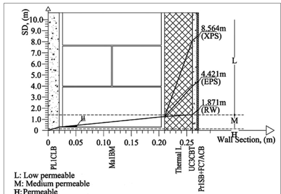
Figure 8. The graph showing the increase in total  $SD$  value throughout the wall section as a function of layer thickness for the walls externally insulated with RW, EPS or XPS, and externally plastered with  $FC7ACB$ . The slope of each line presents the individual  $\mu$  value of each layer.
