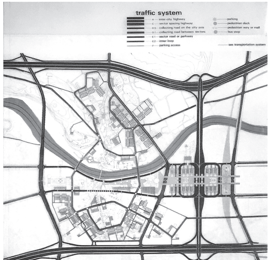
Figure 3. Proposal for Skopje, traffic system. Roads are divided into the categories of function, speed and width. The legend on the upper right corner shows the codes for the categories. (The Kenzō Tange Archive. Gift of Takako Tange, 2011. Courtesy of the Frances Loeb Library, Harvard University Graduate School of Design)
