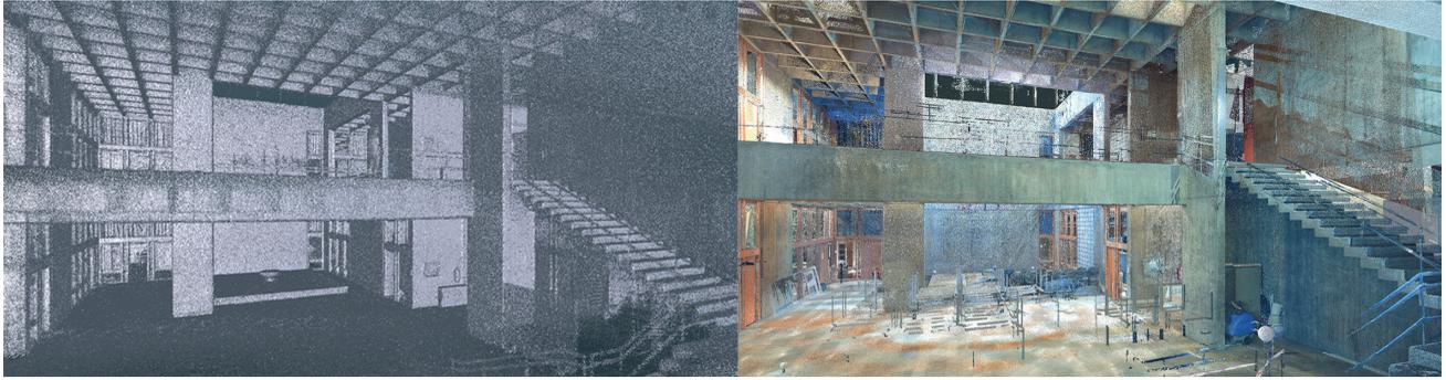
**Figure 7.** Point cloud model scanned with a low precision scanner (left), and with a high precision scanner (right) (Model made by Şahin Akın).
