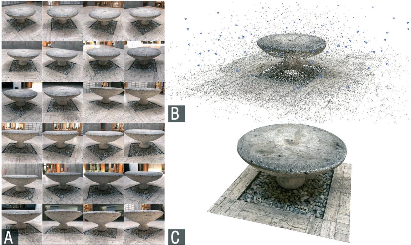
**Figure 8.** A) The photos of the selected geometry, B) Sparse point cloud model, C) Coloured mesh model of the Göbektasi (Model made by Şahin Akın).
