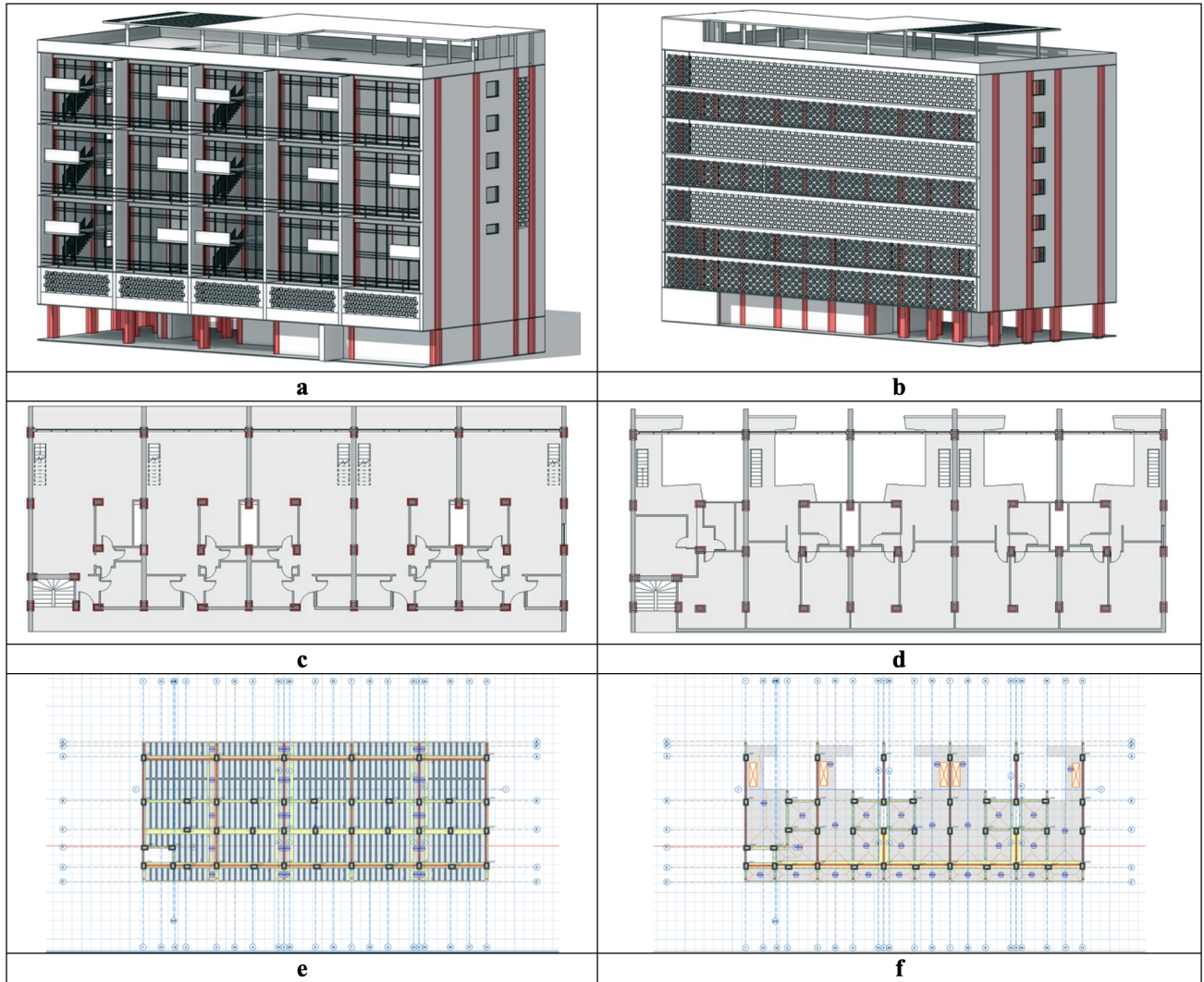
Figure 15. Model 2 – Column-jacketing: a. Perspective views from northwest façade. b. Perspective views from southeast façade. c. Residential unit's entrance floor plan. d. Residential unit's mezzanine floor plan. e. Residential unit's entrance floor ProtaStructure model. f. Residential unit's mezzanine floor ProtaStructure model (3-D images are produced by authors via Autodesk Revit Software; 2-D images are produced via ProtaStructure Software).
